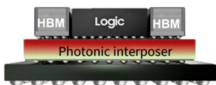
Development trend: Optical interface between HBM and Logic
